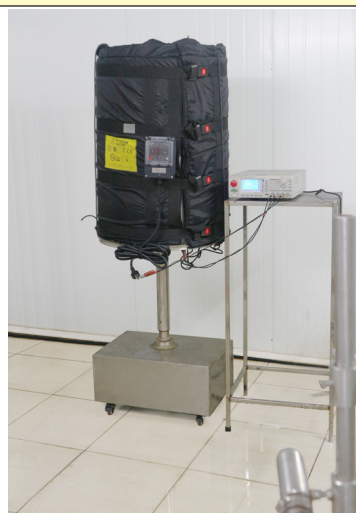
Insulation resistance measurement after IPx6 tests
