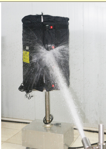
IPx6 testing of jacket heaters
